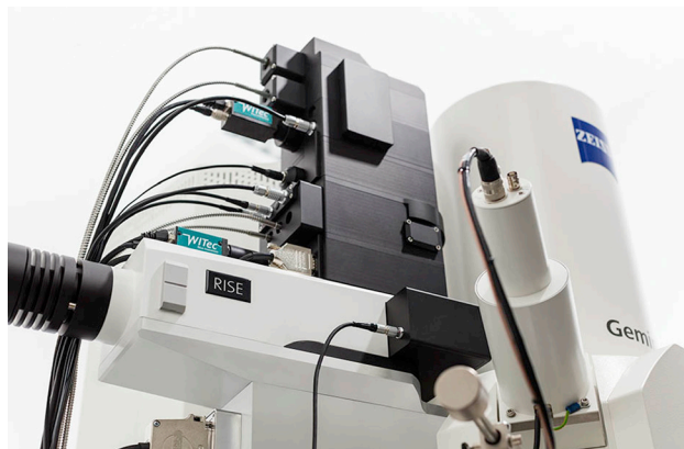
Fig. 1: ZEISS Sigma 300 RISE, a combination of ZEISS Sigma 300 and a WITec confocal Raman microscope
