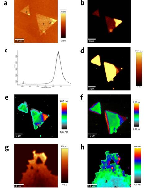
Fig. 3: Correlative AFM-SNOM-PL imaging of WS2
