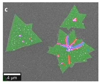
Fig. 2: RISE microscopy of MoS2 crystals
