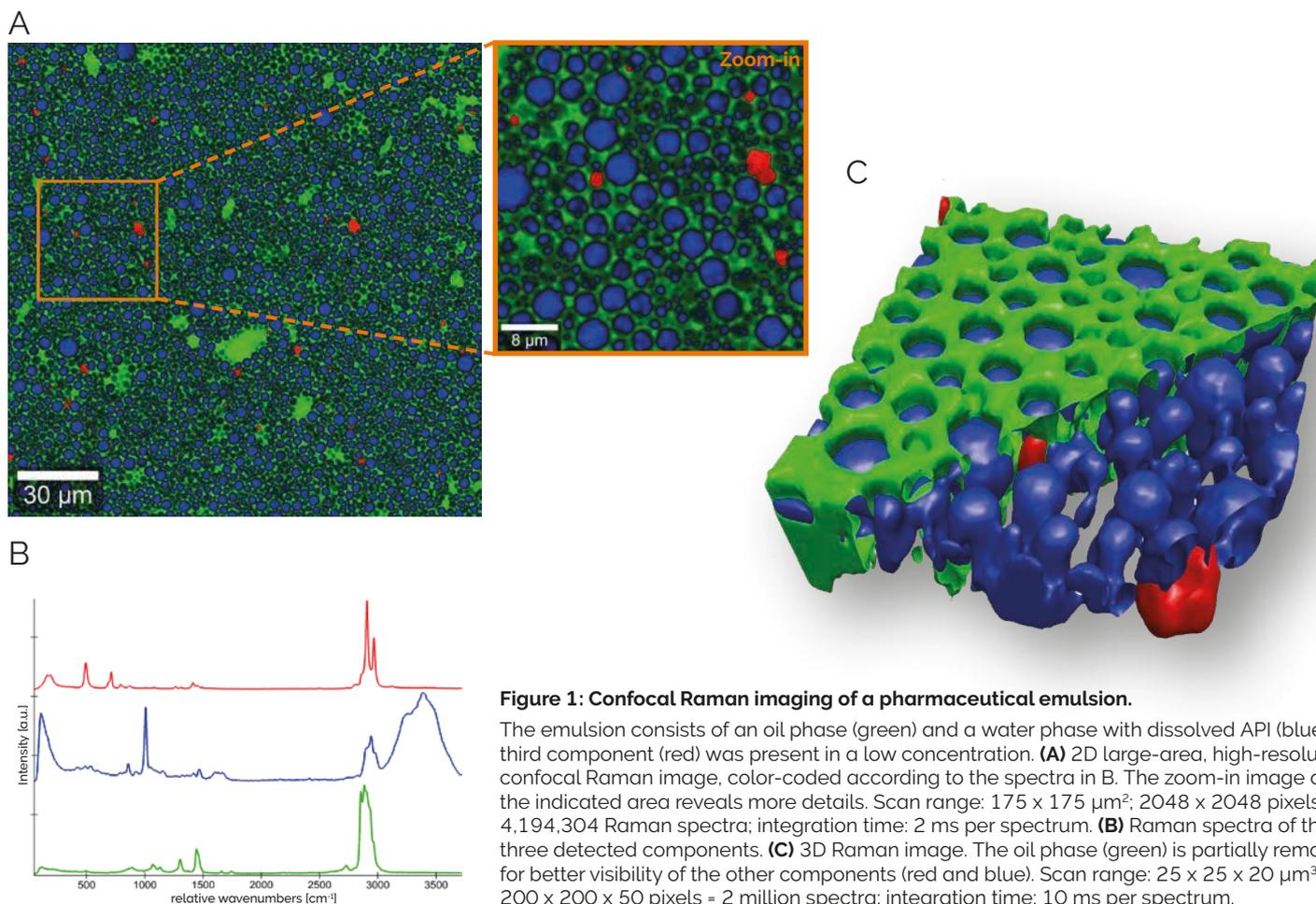
**Figure 1: Confocal Raman imaging of a pharmaceutical emulsion.**
