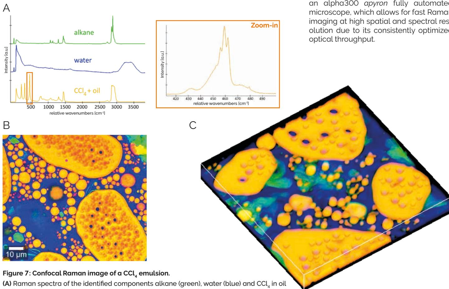
**Figure 7: Confocal Raman image of a CCl<sub>4</sub> emulsion.**
