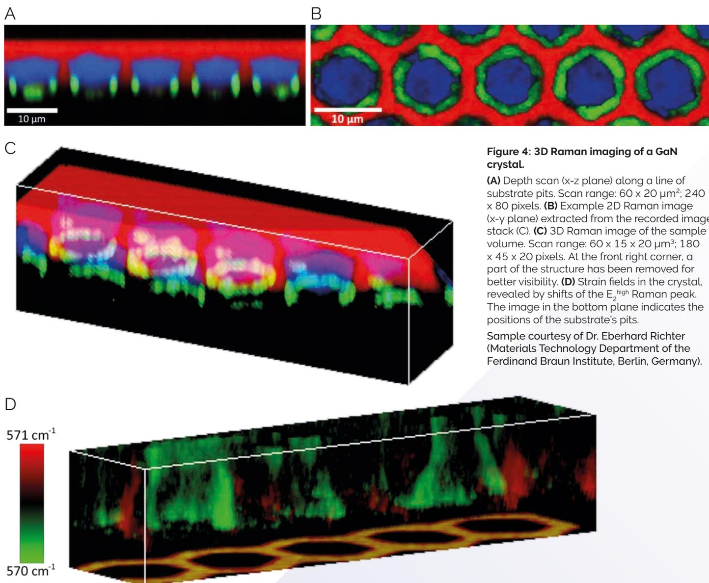
**Figure 4: 3D Raman imaging of a GaN crystal.**
